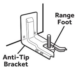
Making sure the anti-tip bracket is installed:
