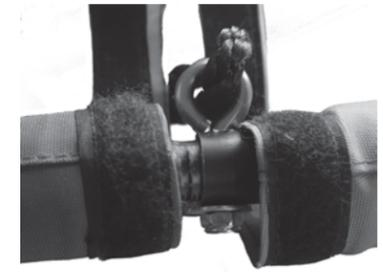
6. Add washer and nut to the bottom side of tube bolt and secure. Tighten with wrench. Repeat both Steps 5 and 6 for remaining three screw ends and hardware.
