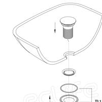
Insert the drain top into the vessel. Install thick rubber washer, 2 O-rings and mounting ring in turn.
