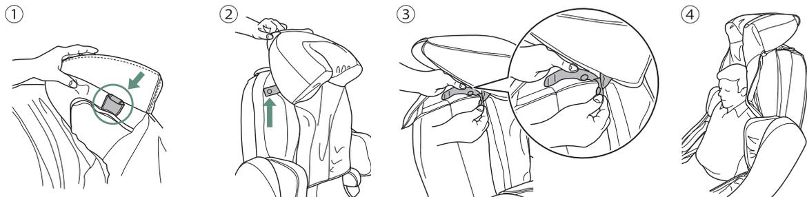
① Flip the side of the Shoulder Massage Unit over, as illustrated. The lock belts for the Shoulder Massage Unit are initially positioned at the rear of the Shoulder Massage Unit.
