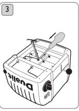
Unscrew brass links and wires.
