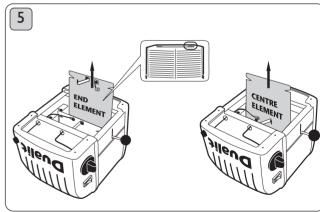
Remove element. To re-assemble, reverse procedure ensuring wires and parts are correctly positioned. Ensure new element is marked the same as the one removed and is seated correctly in the channels either side.
