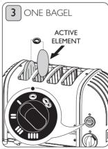
Rotate the 'selector switch' anti-clockwise to the one bagel symbol. Only the second element from the left will heat up.
