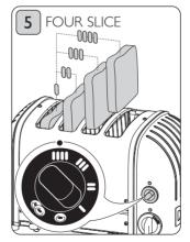
Rotate the 'selector switch' clockwise to the four slice indicator. All slots will heat up.
