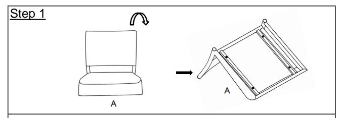
Open the carton, and place all parts onto a clean, non-marring surface. Place the Seat(A) facedown.
