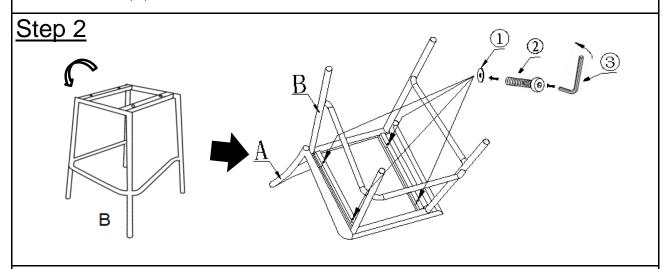
Turn over the Leg Frame(B), and place it onto the Seat(A).
