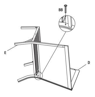
6 Attaching The Metal Plate To The Right Backrest And The Left Backrest
