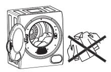
If drying large items such as blankets, it is recommended that you open the dryer door from time to time, shake the items, place them back in the dryer and close the door. This will ensure even drying.
