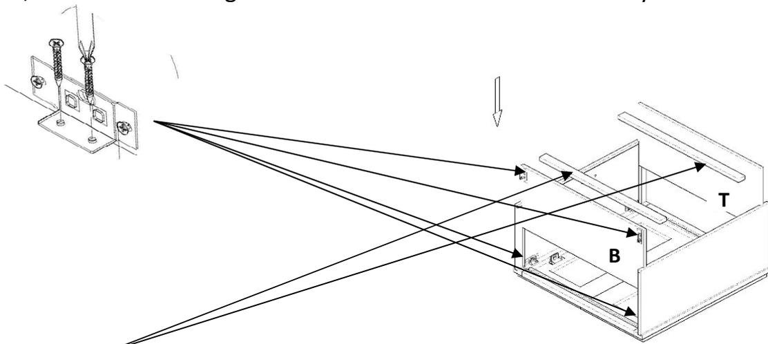
The two optional hanging bars are included. These are to be installed at the top and bottom of the inside of the cabinet prior to mount to the wall. The Larger screws(M 2 3/8") are needed.
