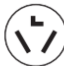
3-wire receptacle (10-30R)
