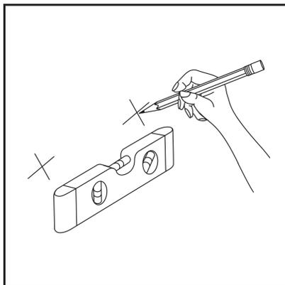
Determine type of wall anchor to use. Type of anchor depends on wall surface and weight of item to be hung. Consult professional if in doubt. Using a tape measure and level, mark position for the anchors. Space anchors so the attached Rings or Keyhole hangers will hang on anchors properly.
