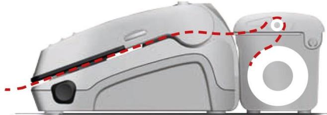
3. Open the top cover of the vacuum sealer and pull the desired length of bag through the slot in the top cover.
