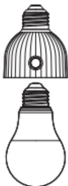
Screw in the E26 base LED bulb into the Smart Socket.
