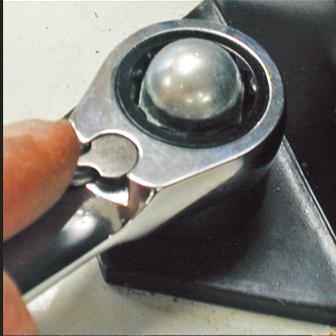
Reversing lever allows you to switch motion from left to right without removing the wrench.
