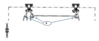
(a) Tie one end of the pull cord to the left front bar of the awning, thread through left side pulley, then over closet right side pulley and down to the cleat and back up to open right pulley, tie the end of pull cord to the right and left side of the front bar. Draw all slack in pull cord towards cleat and tie off. (Shown Below)
