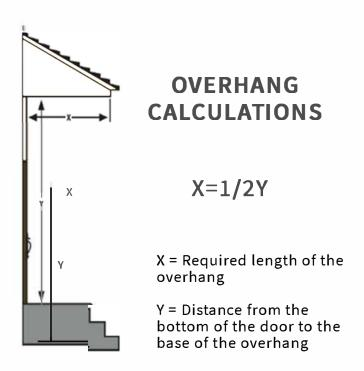
**For example,** if the measurement from the base of the door to the bottom of the overhang is 8 feet, then the required overhang length is 4 feet.
