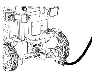
Completely uncoil garden hose or remove completely from reel to prevent kinks.
