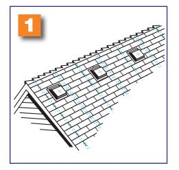
**1. POSITIONING VENTS ON THE ROOF**
