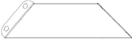
D03 CORBEL - A4M01826 (x1) 2 3/4"x5 11/16"x20 1/16" (70x145x509)
