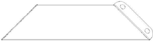
D01 CORBEL - A4M01817 (x1) 2 3/4"x5 13/16"x22 1/4" (70x147x565)
