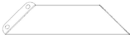
D02 CORBEL - A4M01818 (x1) 2 3/4"x5 13/16"x22 1/4" (70x147x565)
