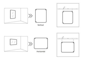
02. Paste the combination template/level on the determined wall, keep the level bead liquid in the middle level to ensure the mirror is level.
