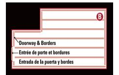
Placement Recommendation: Apply strips to the perimeter of the room, down the center, along doorways and across the interior of the room (see B). Always follow the floor manufacturer's specific installation guidelines.
