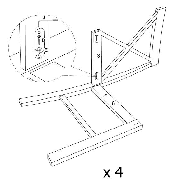
Using bolt (D) insert bent washer (E) secure part (3,6) with hex key (J) as per diagram.
