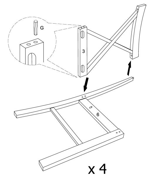
Insert dowel (G) into part (3) attach part (3) to part (6) as per diagram.
