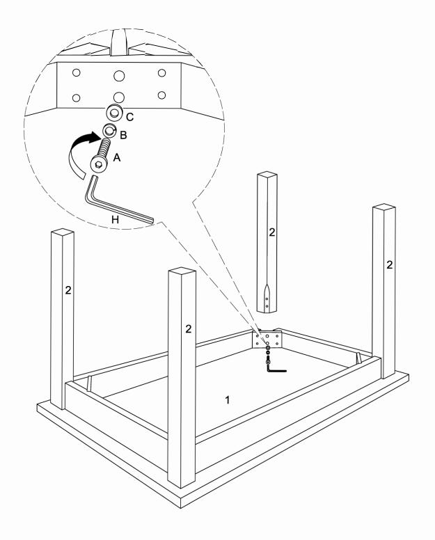
Using bolt(A) connect spring washer (B) and washer (C) to secure top panel (1) to legs (2) with hex key (H) as per diagram .
