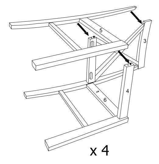
Put part (5) into parts (3,4) as per diagram.
