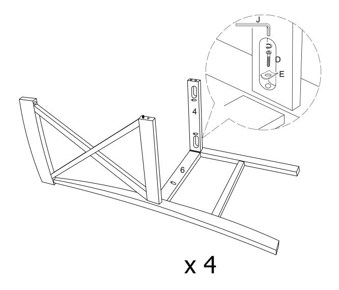
Using bolt (D) insert bent washer (E) into part (4) to part (6) with hex key (J) as per diagram.
