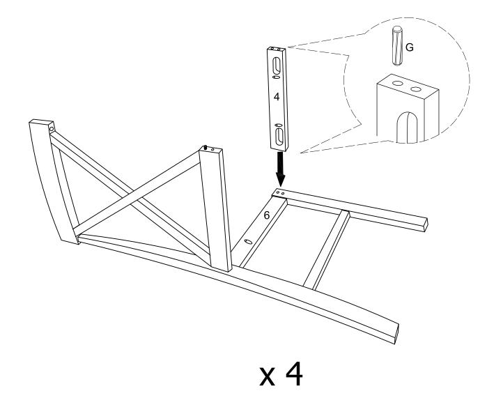
Insert dowel (G) into part (4) attach part (4) secure to part (6) as per diagram.
