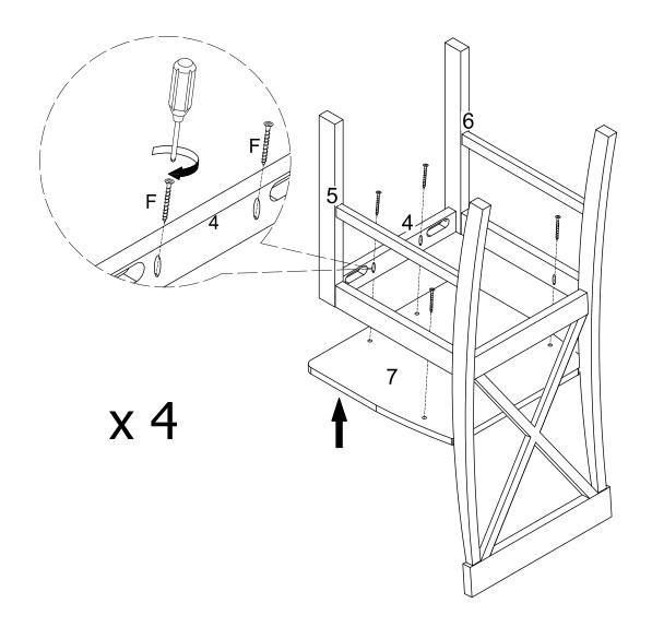
After full adjustment, secure part (7) to parts (4,5,6) with screw (F) and a Philips Head screwdriver as per diagram .
