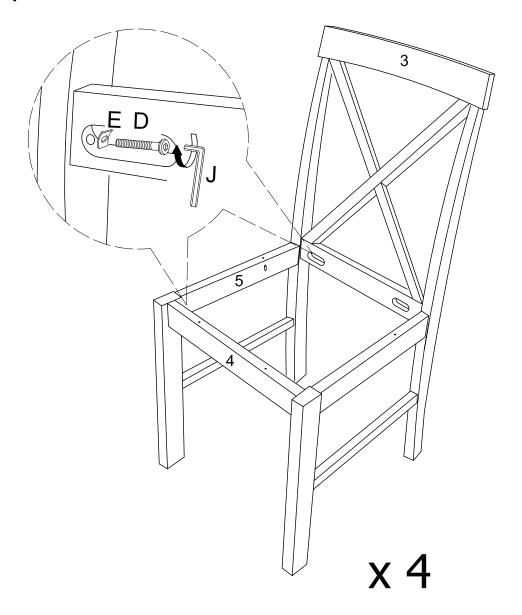
Using bolt (D) insert bent washer (E) secure part (3,4,5) with hex key (J) as per diagram. Please do fully tighten all the bolts .
