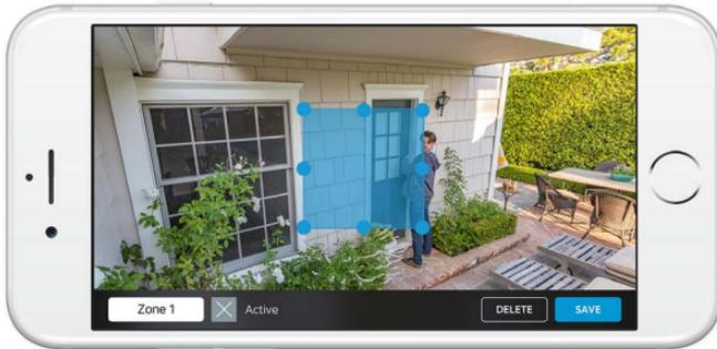
To receive Motion Alerts, set up one or more Motion Zones. These are customizable areas of the camera view that you select for motion detection. If motion occurs in one of your Motion Zones, you're sent a Motion Alert.
