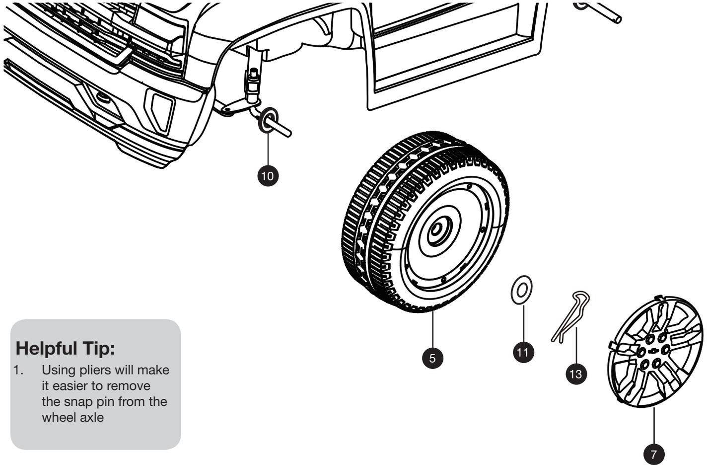
1. Locate the  $\Phi 10$  Thick Washers (10), the  $\Phi 10$  thin washers (11), and snap pins (13) from blister pack.
