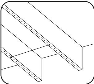
**Note:** Measure from center to center of ceiling joists using a tape measure.
