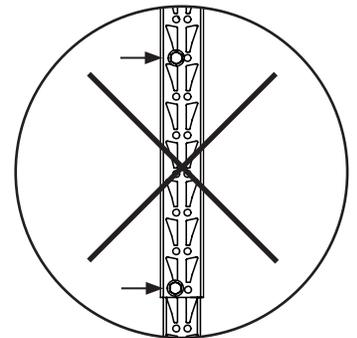
**Note:** Must be bolted at the highest point and lowest point of the two posts and at opposite holes.
