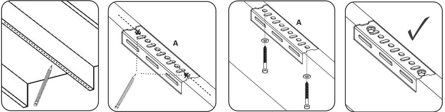
**!** *Note: Install into solid wood joists only. Brackets must be mounted perfectly in line and square to each other. Make sure the lag bolts are tight against the joist but DO NOT over-tighten the lag bolts. If they are over-tightened, the bolt could snap or the hole may be stripped.*
