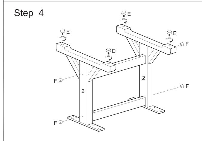
Screw feet (E) into leg pieces (2). Insert wood buttons (F) into leg pieces (2).
