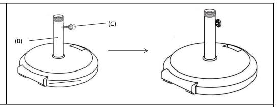
Screw Adjustable Screw(C) into Support Pole(B).
