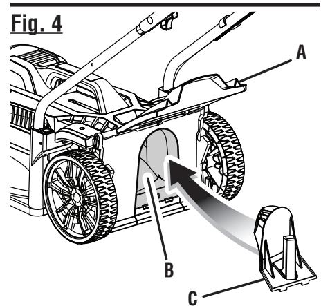
A - Rear discharge door (couvercle d'éjection arrière, puerta de descarga posterior)
