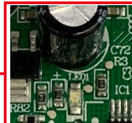
LED1: Drive failure indicator
