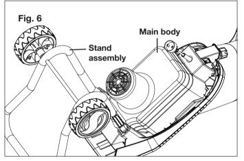
**2.** Align the holes on the main body housing and stand assembly, insert the washer into the screw and install into the stand assembly on both sides (Fig. 7).
