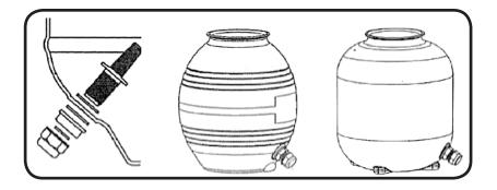
2. Press and turn the sand tank to mount it to the sand filter support with correct direction, drain plug on the outside (see below)
