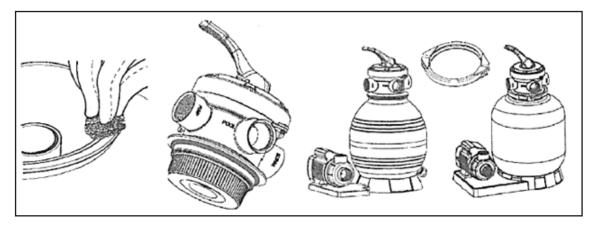
5. Connect the sand tank to the pump with hose and hose adapters.
