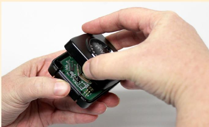
**Step 1:** Push in the latch panel on the bottom of the door sensor and lift the top to remove it.
