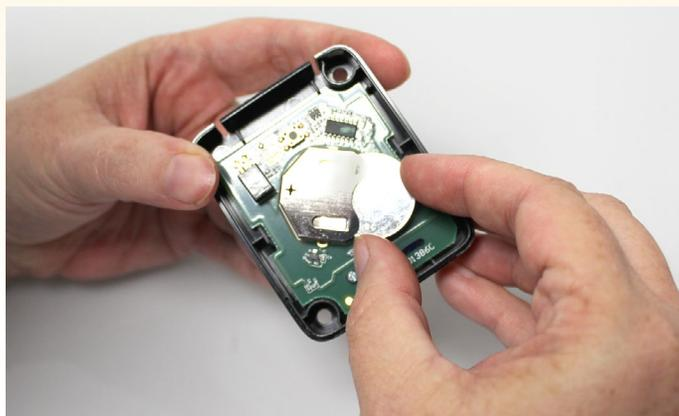
**Step 3:** Gently but firmly insert the new battery into the clip and replace the cover.
