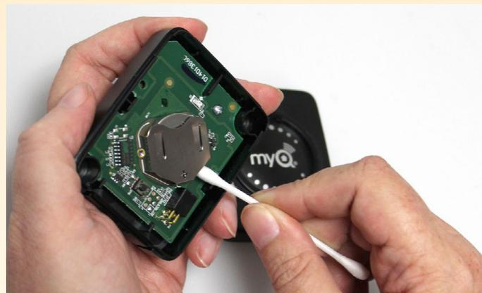
**Step 2:** Using a soft nonconductive tool (such as a cotton swab), gently push the coin battery out of the clip.
