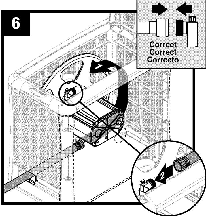
Pull garden hose around the hose reel and connect to out-tube.
