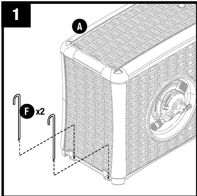
Secure crate (A) to ground with two stakes (F) using a hammer.
