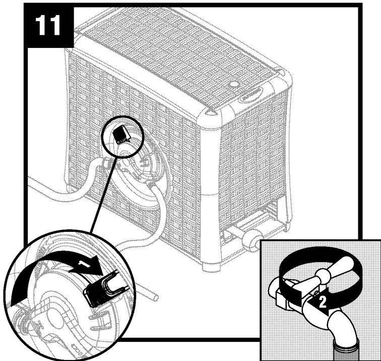
Move lever to the rest position and turn off water.
