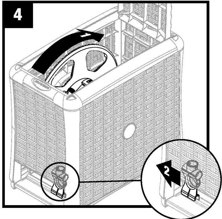
Lift crate lid and manually rotate hose reel until the SmartTrak™ hose guide is in the left most position.
