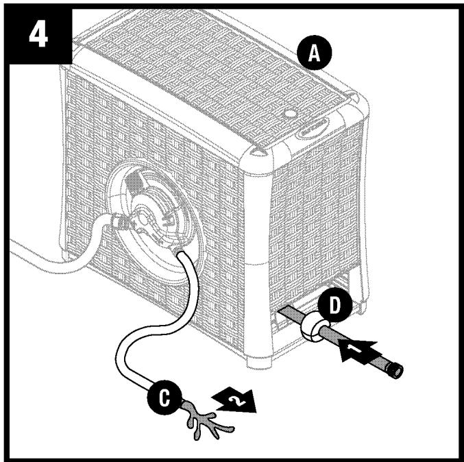
If necessary, guide hose during rewind. Rewinding will stop when hose stopper (D) hits crate (A). Move lever to the rest position and turn off water.
