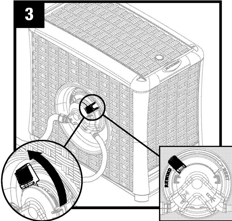
To roll up hose, move lever to rewind position.
