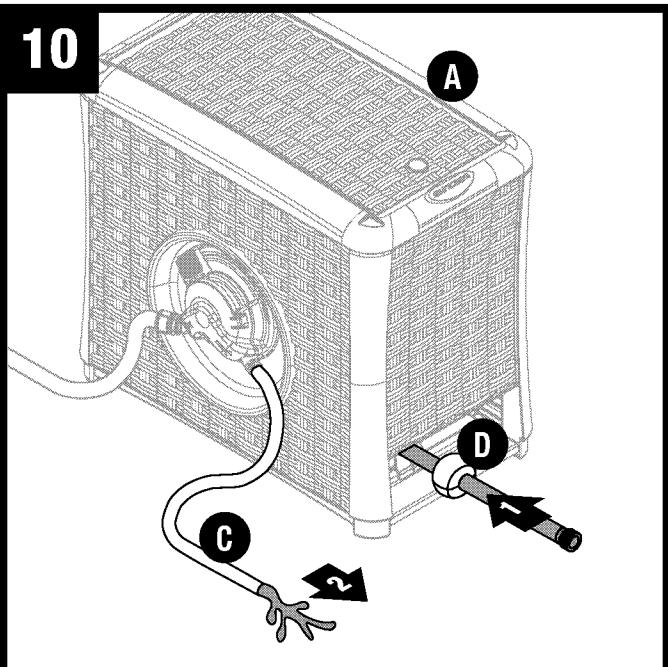
Approximately 4-6 gallons of water will be discharged from the drain hose (C) during rewind. If necessary, guide hose during rewind. Rewinding will stop when hose stopper (D) hits cage (A).
