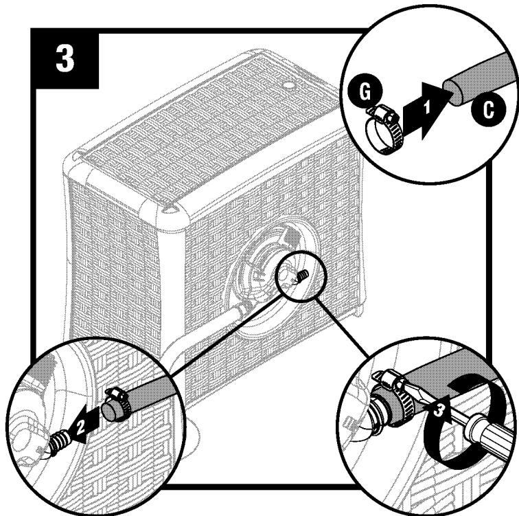
Attach hose clamp (G) to drain hose (C). Connect one end of drain hose to drain hose outlet. Tighten hose clamp with flat head screwdriver. Place the other end in a suitable water drainage area.
