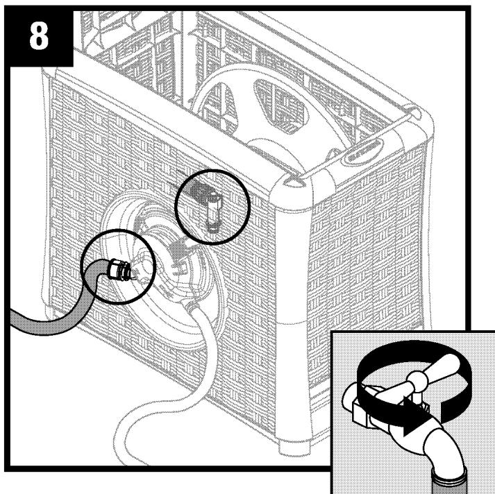
Attach hose nozzle (not included) to male end of garden hose. Attach hose stopper (D) with two screws (E).
