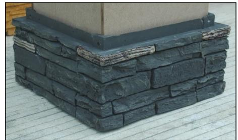
**3)** Each box contains 2 left (L-2,L-4) and 2 right corners (R-1, R-3). 2 boxes are needed per 2 courses. Use 4 right pieces for 1 course and 4 left pieces for the next course. Dry fit corners R-1, R-3 and R-1, R-3. Slide down onto the starter strip and attach all pieces where indicated on the screw hem.
