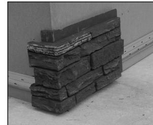
**Note:** There are 4 patterns of the Slatestone Outside Corner. 2 Left patterns and 2 right patterns. Check for numbers on the backside of the piece. They are numbered 1 through 4. Alternate left and right corners with each course to prevent pattern repetition.
