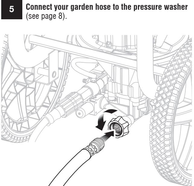
Completely uncoil garden hose or remove completely from reel to prevent kinks.
