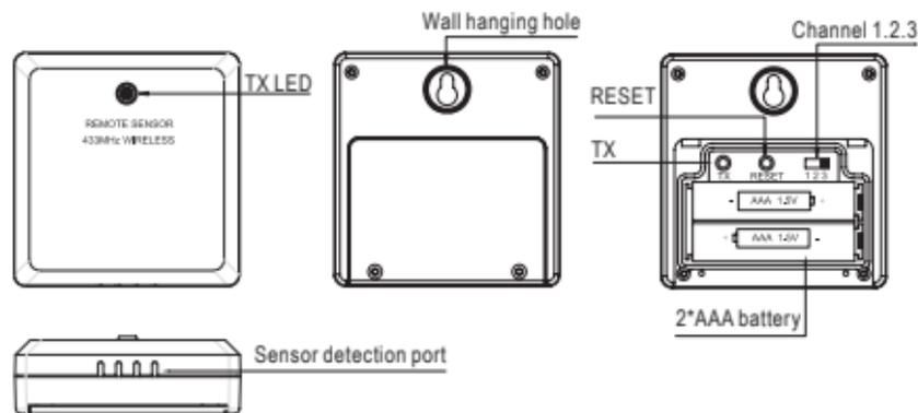
1. Battery Compartment: Holds 2 X AAA batteries to power the unit.
