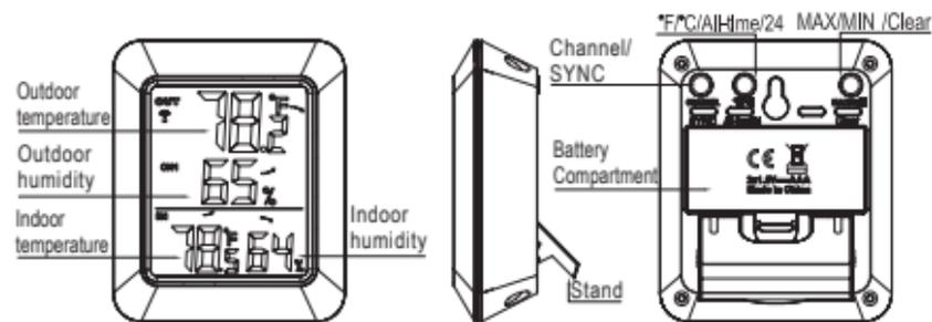
1. LCD display: Displays the current outdoor humidity/temperature and indoor humidity/temperature.
