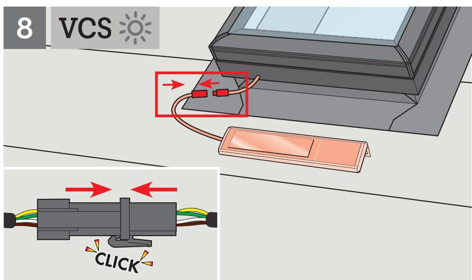
**ENGLISH:** For VCS: You are now ready to install the flashing. If the flashing is not to be installed immediately, install solar panel and reinstall cladding.
