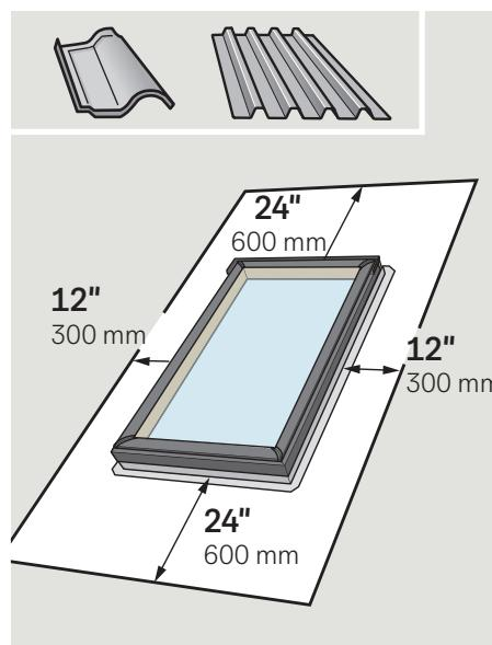
**ENGLISH:** Maintain illustrated clearances between skylight frame and critical areas such as valleys, ridges, slope changes and roof-to-wall-intersections.
