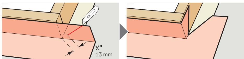
**ENGLISH:** To ensure waterproofing, skylight curbs should be completely wrapped in VELUX adhesive skylight underlayment as indicated. This underlayment must be applied before installing the flashing.
