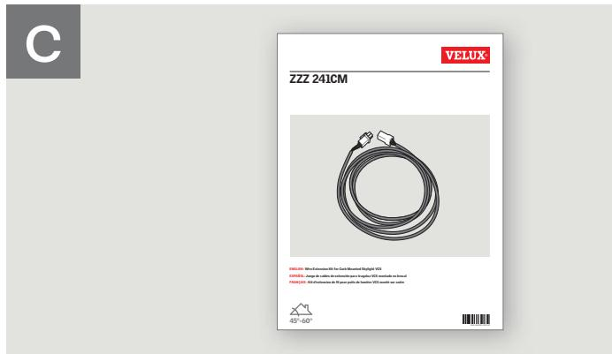
**ENGLISH:** For steep roof pitch above 30° (6:12) use wire extension kit ZZZ 241CM to relocate the solar panel and rain sensor as shown in the enclosed instructions for ZZZ 241CM.
