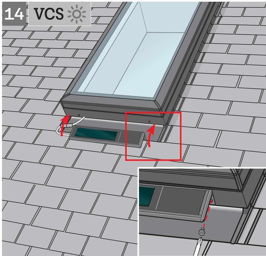
**ENGLISH:** Install solar panel as shown and secure with screws.
