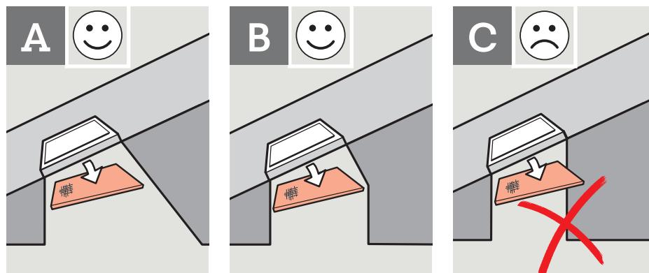
**ENGLISH:** For skylights provided with an insect screen, a flared light shaft is required to remove the insect screen. See details.
