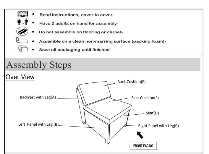
This Armless Chair has multiple parts and may require up to 30 minutes to assemble. To give you an overview of the Armless Chair parts, the above picture is to help you put the various parts into perspective. Please read through the instructions below to familiarise yourself with the parts and steps before assembly.
