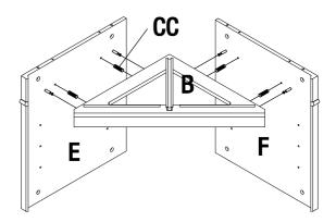
□ e) Connect the fixed panel (B) and panels(E/F) with cam lock(AA).
