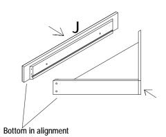
$\Box$  d) Fix panel(J) by tightening screws(FF).
