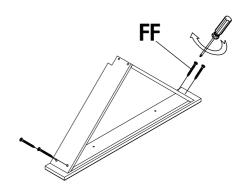
□ e) Assemble drawer glide(0) to drawer bottom with screws(FF).
