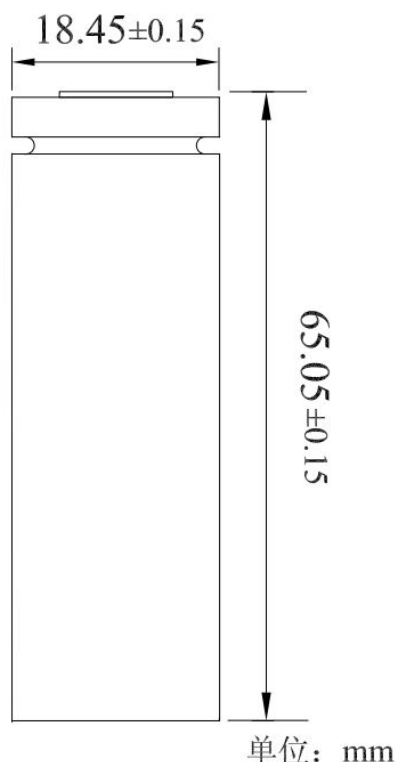
Fig.1 Outline Dimensions of CMICR18650F8-2600mAh(with tube)
