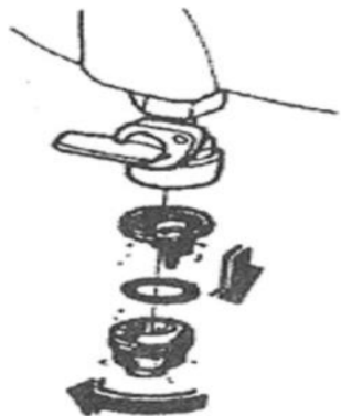
FUEL FILTER ELEMENT REMOVAL
