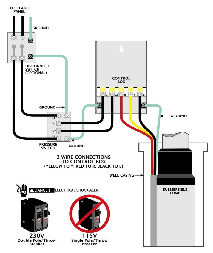
Typical connection--- connect with 4" deep well pump
