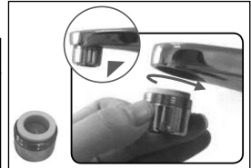
Figure 9 - Aerator Installation (3kW Models ONLY)
