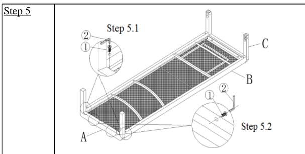
**5.1**) Attach Front Leg(C) to Seat Panel(B) using Bolts(1) with Allen Key(2) as shown above.
