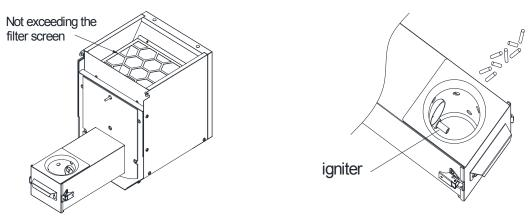
The device begins to ignite. White smoke will be emitted during the ignition of the fuel, and personnel can stay away from the operating device before the completion of the ignition.
