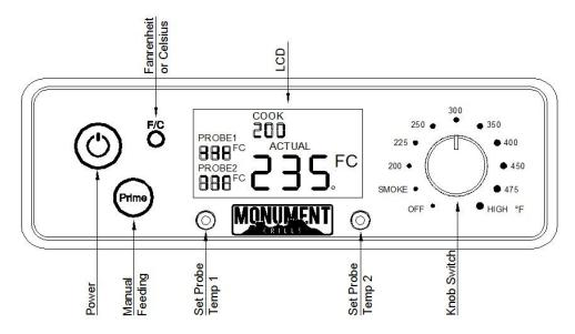
(少) This is the power button of the device(Power indication function included).
