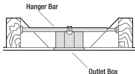
To hang your fan where there is an existing fixture but no ceiling joist, you may need an installation hanger bar (not included) as shown above.
