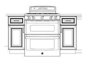
Make sure to give landing space on each side of a cooking appliance when placing in design.
