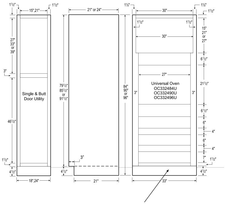
NOTE: 96" TALL CABINETS ARE SUPPLIED WITH LOOSE TOE KICK BOX (EXPOSED SIDES REQUIRE TSK96)
