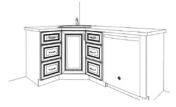
For sufficient dishwasher door clearance and loading/ unloading space, a 15" wide base cabinet is recommended for use between a corner sink base and dishwasher.
