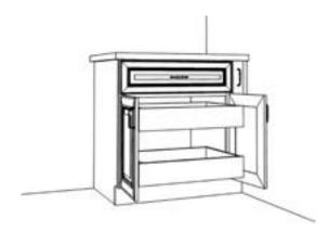
Be sure to leave enough clearance for doors to open at least 90 degrees. This will allow the roll out trays to be operated correctly.
