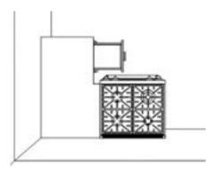
When placing a blind base cabinet, cabinet with drawer or trash pull out, make sure to allow enough clearance so drawer/pull out will open fully.
