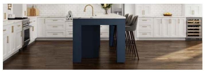
Need a nice square post for your island, or want a raised bar? Use fillers to create a square post to the width and height of your choosing. This image uses 6" wide fillers, however 3" wide fillers can be used as well. To create the apron under the countertop turn fillers horizontally and cut to fit on the job site.
