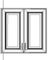
When placing cabinets against a side wall, use a minimum of 3/4" filler between wall and cabinet to allow doors to open
