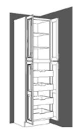
Make sure to leave enough clearance for door to open at least 90 degrees when placing next to wall or refrigerator cabinet.
