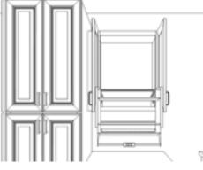
Make sure to allow proper clearance on each side so doors can open 90 degrees or more. This will allow the interior accessory to pull down correctly.
