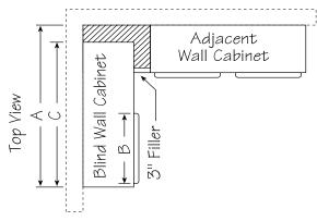
**BLIND WALL INSTALLATION GUIDE** Wall Space "A" Frame Opening Cabinet Width "B" Width "C" Cabinet Min - Max WBCU2730 25" - 30" 8<sup>7</sup>/8" 24" WBCU2736 25" - 30" 8<sup>7</sup>/8" 24" 25" - 30" 8<sup>7</sup>/8" 24" WBCU2742
