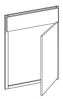
Most Base cabinets can be ordered as "Cabinet Fronts Only". Face frame, doors, drawer fronts, hinges, and bumpers will be supplied and shipped loose. In addition, plastic corner blocks will be supplied for false front installation requirements.
