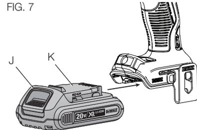
handle until the battery pack is firmly seated in the tool and ensure that it does not disengage.
