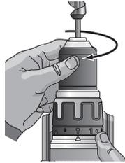
Be sure to tighten chuck with one hand on the chuck sleeve and one hand holding the tool for maximum tightness.
