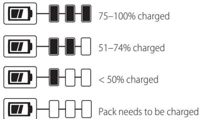
To actuate the fuel gauge, press and hold the fuel gauge button. A combination of the three green LED lights will illuminate designating the level of charge left. When the level of charge in the battery is below the usable limit, the fuel gauge will not illuminate and the battery will need to be recharged.
