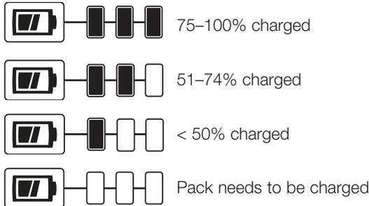
To actuate the fuel gauge, press and hold the fuel gauge button (L). A combination of the three green LED lights will illuminate designating the level of charge left. When the level of charge in the battery is below the usable limit, the fuel gauge will not illuminate and the battery will need to be recharged.
