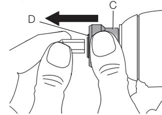
**To install an accessory,** fully insert the accessory. The accessory is locked into place (Fig. 6).
