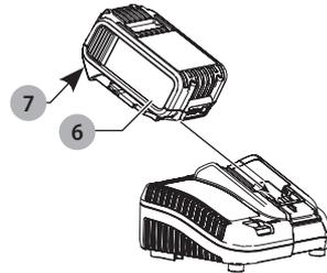
2. Insert the battery pack **6** into the charger, making sure the battery pack is fully seated in the charger. The red (charging) light will blink continuously indicating that the charging process has started.
