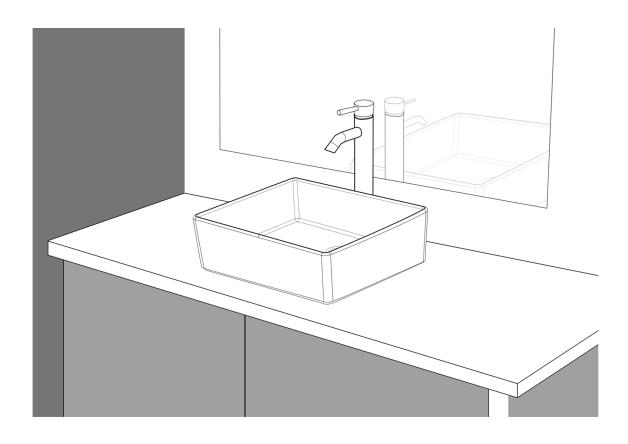
Step#2: Once the position is confirmed, mark the center of the drain hole and set aside the vessel sink. Draw a 3 inch diameter circle around the center of the drain hole. Use a jigsaw or a power tool to cut the opening on the countertop.
