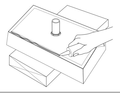
Step#5: Install the sink well and connect P-trap to the drain and check for alignment. Apply some caulking around the base of the sink to seal any gap between the sink and the countertop.
