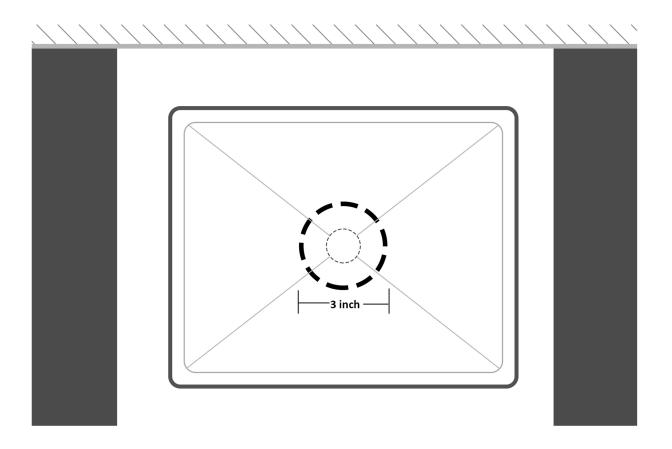
Step#3: Install drain according to manufacturere's installation instructions.(Note: drain not included, and do not overtighten the drain, which will damage the sink surrounding area.)
