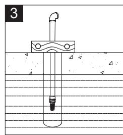
4. Remove pipe clamp and slide a well seal (not included) over the PVC pipe and onto the well casing (not pictured). The PVC pipe should extend approximately 12 in. from the well seal, depending on the height of the pump (A).
