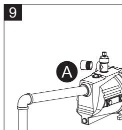
10. Wrap all threads with thread tape. In order for the pump (A) and the pressure tank (not included) to operate properly, the pressure tank needs to be drained of all water BEFORE INSTALLING ITTO THE PUMP. Thread a 10 in. tank tee (not included) or another necessary size tee into the pressure tank.
