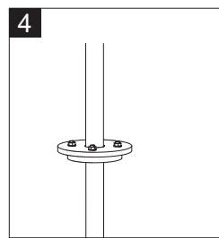
**NOTE:** DO NOT let the assembly slide down into well. Tighten the well seal until the rubber gaskets are tight against the well casing and the PVC pipe.
