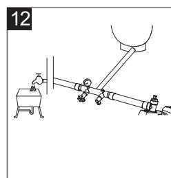
**CAUTION!** Never install a shut-off valve between the pump (A) and the tank, as this can cause excessive friction loss and can damage the pressure switch and/or pump (A). If necessary, only install a fully open gate valve (not included).
