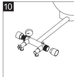
11. Air pressure in the tank must be 2 PSI lower than the "cut-in" of the pressure switch.
