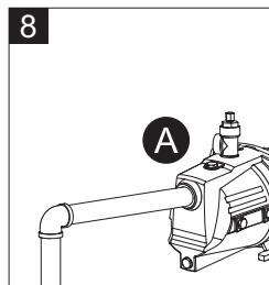
9. Wrap thread tape (not included) around the threads of a 1 in. male PVC adaptor (not included), and thread the adaptor into the discharge tee.
